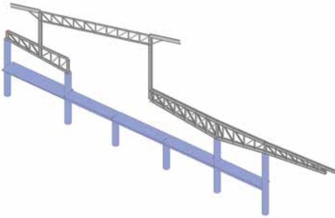
Figure 7. Low roof truss supporting high roof—RISA 3D model.
